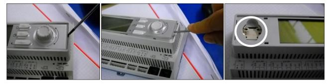
Be careful to avoid damages to the plastic cover. The new battery shall be placed in the proper battery holder which is highlighted in the following picture, respecting the polarities indicated into the holder itself.
