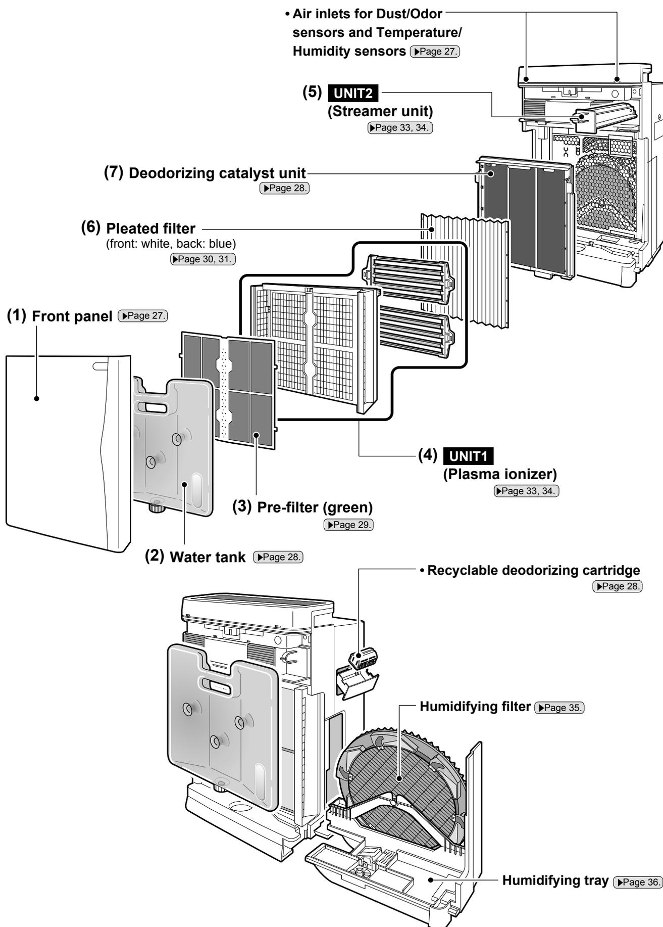
To clean the humidifying tray or humidifying filter, first remove the (1) front panel and remove the (2) water tank.
