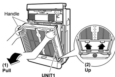
**4** Remove the opposite pole plates on the backside of UNIT1.
