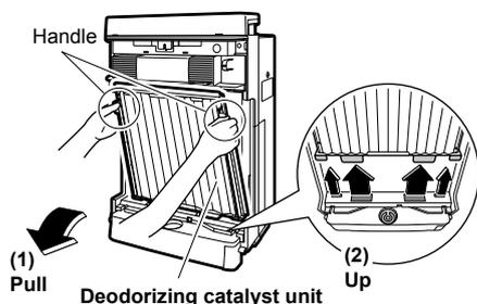
**5** Replace the plated filter with a new filter.
