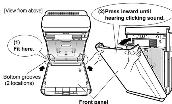
To correctly restore the front panel, press the front panel until hearing the clicking sound from the left and right sides. Unless properly installed, a safety switch may trip and prevent the unit from starting. ▶Page 27.
