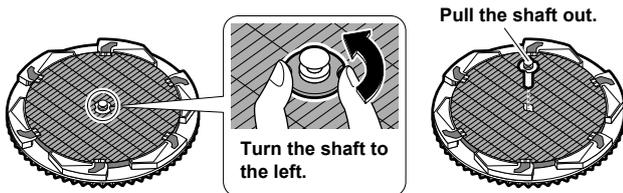
**4** Remove the humidifying filter from the waterwheel, and attach a new filter.
