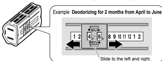
(When the left slot is over the starting month, the month that the deodorizing cartridge should be regenerated is shown in the right slot.)
