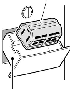
Use to regenerate the recyclable deodorizing cartridge. Inserting into the streamer pocket decomposes absorbed odors and enables reuse.
