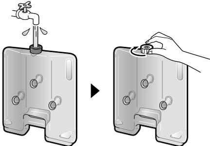
Close the water tank cap tightly.
