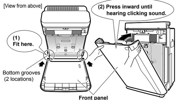
To correctly restore the front panel, press the front panel until hearing the clicking sound from the left and right sides. Unless properly installed, a safety switch may trip and prevent the unit from starting. ▶Page 27.
