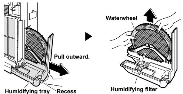
Do not remove the humidifying filter from the waterwheel. The filter may lose its shape.
