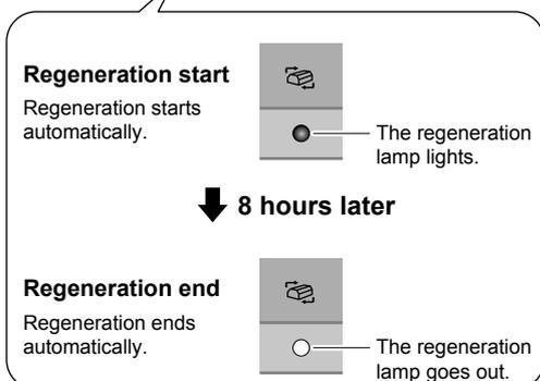
After regeneration ends, remove the recyclable deodorizing cartridge and return it to its place of use.
