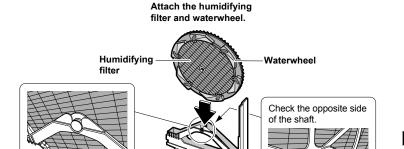
Install the humidifying filter and waterwheel in the direction shown in the figure.
