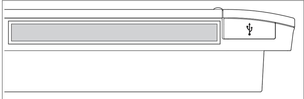
[ψ] Pulling up the rubber cover reveals a USB socket. This socket can be raised 90 degrees, so you can plug in a USB device to it from the front direction when there is no clearance from the side edge of the unit.
