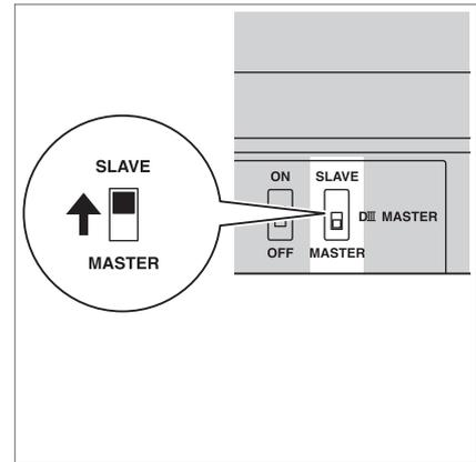
To install multiple centralized controllers, set only the highest priority controller to MASTER and all other controllers to SLAVE according to the following order of priority:
